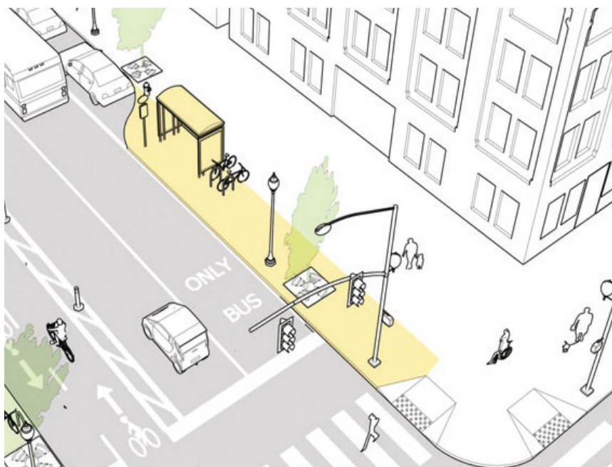
Bus bulbs are curb extensions that align the bus stop with the parking lane (Image: NACTO, 2013b).
